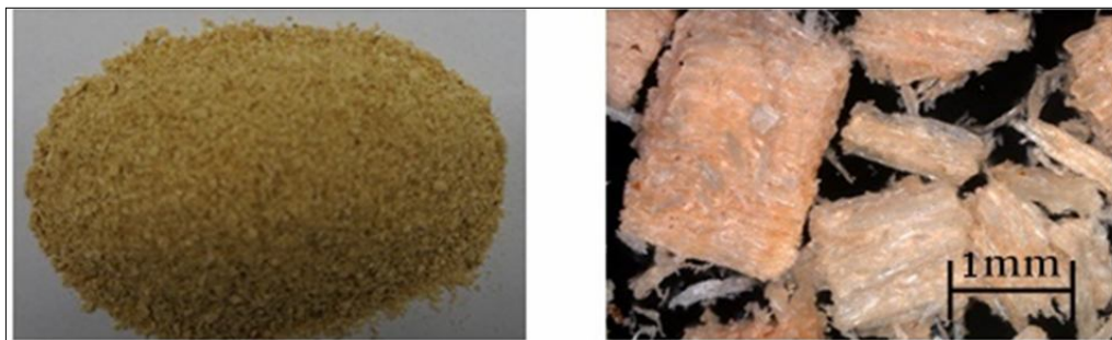
Figure 2. Beech sawdust with particle size < 2 mm; (left) optical camera; (right) optical microscope: Zeiss AXIO Imager.M2m.
