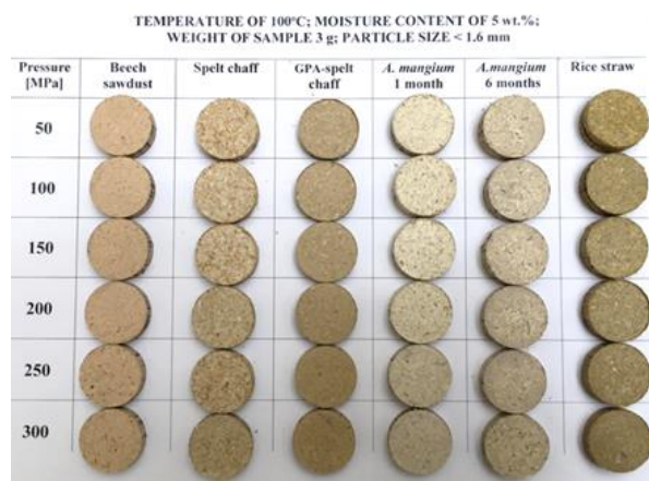
Figure 7. Biomass tablets are produced from different raw materials and under different pressures.
